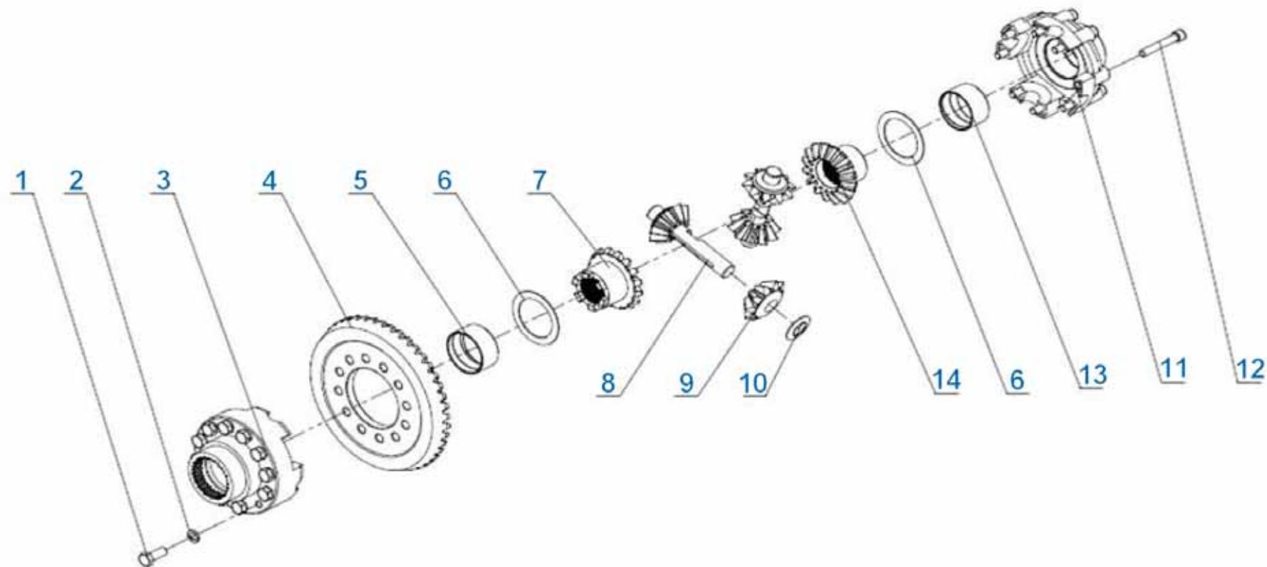
**Differential mechanism assembly list**
